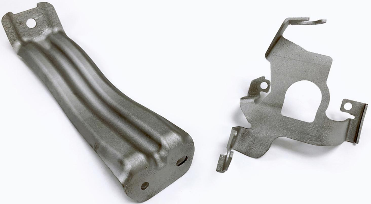
Automotive 3D printed serial parts made on the EOS M300-4 as part of the IDAM project.
