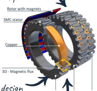
3D magnetic flux design for best weight / performance ratio
