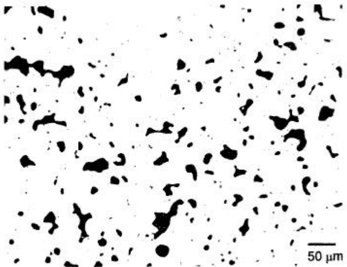
Figure 16: Microstructure of Sintered TRS Bar (composed of 410L with 1 w/o coarse Ancor GS-6000)
