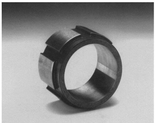
Binder Treatment Process: Binder Treatment Benefits: Farm Tractor Transmission sleeve Burgess Norton Mfg. Co. John Deere FLC-4608 sinter-hardened 6.8 g/cm<sup>3</sup> 75% more effective than wrought steel. Significantly improved reliability ANCORBOND Improved finish by eliminating galling during ejection.
