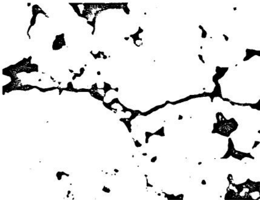
Figure 24: Artificial defect produced by compacting a partially filled die at 25 tsi, completing the fill, and final compaction of the entire part at 45 tsi.
